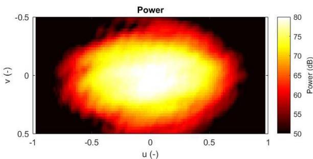
Fig. 5. Two-way gain of QR77SAW, from characterization measurement.
