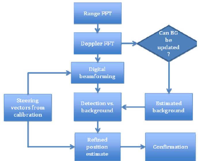
Fig. 3. Block diagram of signal processing in the radar (excluding tracking function).
