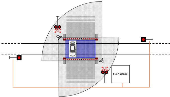
Fig. 1. Schematic illustration of a level crossing. The road runs from top-to-bottom, and the railway from left-to-right. In this example a car is shown obstructing the railway, even though the barriers are closed. Two sensors (radars) are illustrated on opposite corners, which are combined to control the level crossing (denoted FLEX-control), which could then activate signals at some distance from the crossing to warn approaching trains.
