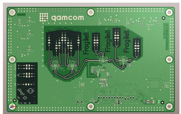
Fig. 2. Picture of the radar front-end, showing the positioning of the transmitter antennas (Tx) and receiver antennas (Rx).
